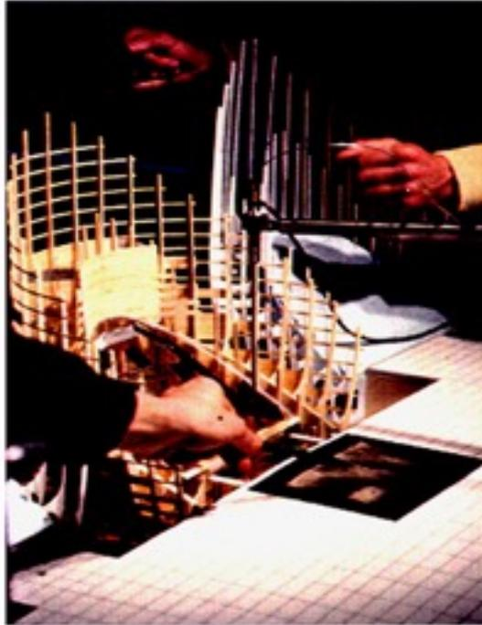
MAQUETTE D'ESSAIS PRESSION AU VENT C.S.T.B.
